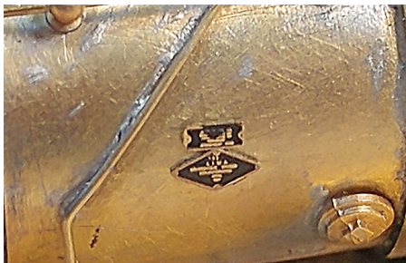
Figure 192: A tiny drop of epoxy was placed on the smoke box in the center of each builder's plate location. Each plate was allowed to fully cure before the next was applied.
