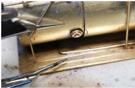
Figure 190: This is one of the few times that I did not use Dykem for marking brass. As I could not adhere the parts without removing the coloring it made no sense to use it. Instead I relied upon two very light scribe marks made in the brass.
