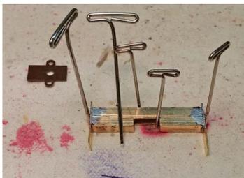
Figure 38: The end caps were held in place with T pins while being soldered. After filing and smoothing, the end caps were scored with a saw just like the face of the beams.
