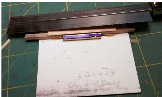
Figure 37: One of the end beams in the scoring jig.
