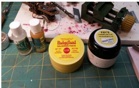
Figure 34: These are the solder flux products used for this installment. From left to right: Tix Flux and Anti Flux, Rubyfluid, and Fry's.
