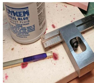
The main body of the end beams was cut from 1/8" x 1/4" rectangular brass tube. (Figure 36) Using a simple jig, I scored the middle of the tube lengthwise to create the appearance of two separate parts joined together. (Figure 37)
