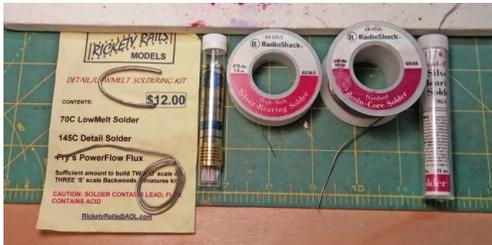
Figure 33: The six solders used for making the end beams. From left to right they are two detail solders from Rickety Rails, Tix stick solder, a 62/36/2 silver bearing solder, a 60/40 solder, and a 96/4 silver solder.
