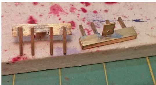
Figure 42: All eight foot board hangers soldered to the end beams.
