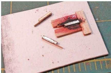
Figure 40: The assembly jig for the floor board hangers.
