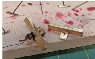
Figure 39: Coupler mounting plates were made of 0.032" by 1/4" brass strip. They were drilled and tapped, as seen here, and fitted with couplers and draft boxes.
