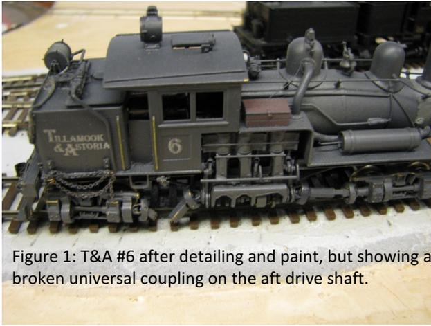
Figure 1: T&A #6 after detailing and paint, but showing a broken universal coupling on the aft drive shaft.
