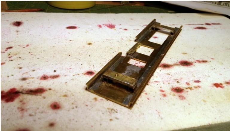
Figure 2: The new Shay frame base plate with side channels, bolsters, and the start of an engine mount soldered in place.
