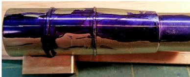
Figure 111: The top center of the boiler was scribed into a coating of marking dye. This was used as a guide for the mounting holes that were later drilled through the boiler and for placing other details on the boiler.
