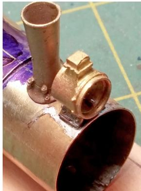
Figure 112: Once soldered in place, I removed the screw inside the smokestack as it would interfere with future work planned for inside the boiler. The screw was only used to hold the stack in place for soldering.
