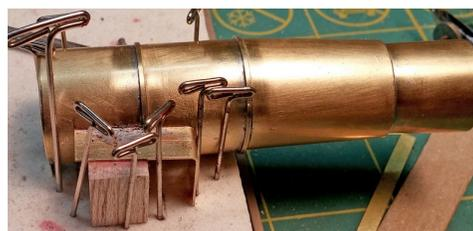
Figure 107: It took several tries to get the engine shroud properly positioned on the side of the boiler. Shown here is my first attempt, which was obviously not right. The boiler tended to roll while the shroud would frequently fall away.
