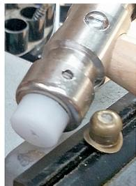
Figure 114: I used both the plastic jaws of my vise and the surface of my cutting mat as a means of gently flattening the curves on the bottom of the steam and sand domes. Shown is the 4 ounce mallet used (Micro-Mark #83434). The nylon head did not mar the brass.
