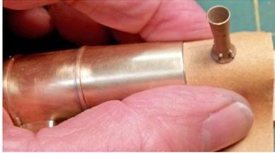
Figure 109: Holding a piece of 220 grit sandpaper over the smoke box, I sanded the bottom of the smokestack (Precision Scale Company #31448) until it matched the curve of the smokebox.
