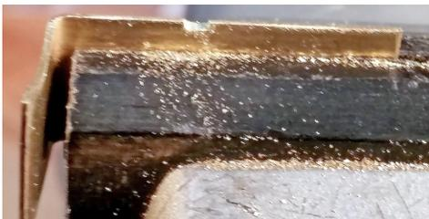
Figure 106: Once trimmed to length, the boiler shroud was notched to accept the boiler band that passes beneath it. The sides of the cut were notched with a jeweler's saw, and then the slope between the notches was filed down with a small square file.
