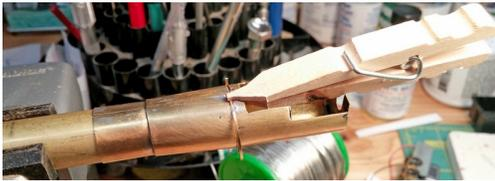
Figure 104: Here one of the boiler bands is held in place by a backwards clothespin clamp. Note: the jaws of the clamp were trimmed down to a narrow tip to allow them to fit in the close quarters of the boiler's underside.
