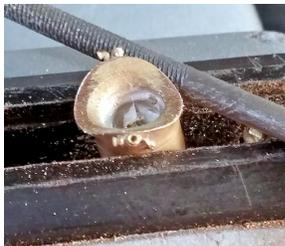
Figure 115: The sand dome was sloped, but naturally it did not match the slope of my boiler. I adjusted its slope with a wide oval shaped file and then finished matching the curves with sand paper as I did with the smoke stack. The sand dome is Precision Scale Company # 32385.
