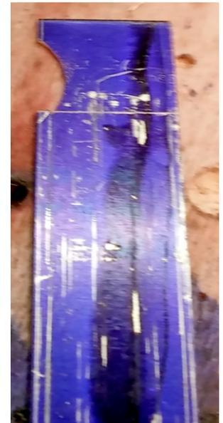
Figure 105: Shown here is the engine shroud while still a flat piece of brass. The curved cutout matches the diameter of the boiler and was traced from one of the card stock patterns made during installment 10 of this series.
