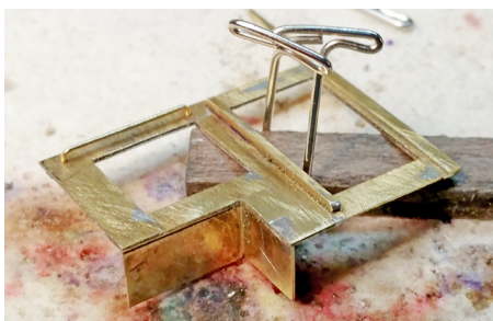
Figure 211: This small brake is suitable for making small parts. I recommend keeping the working piece hard up against the brake's side frame. This helps insure that your bends are perpendicular to the length of the part.
