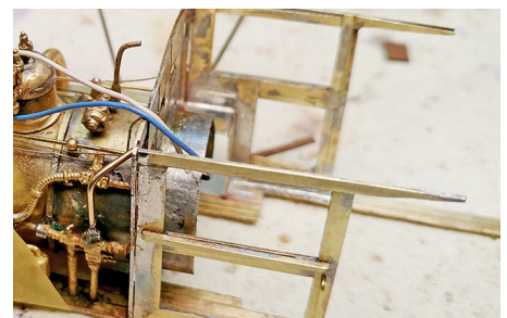
Figure 212: A simple and temporary jig was used to hold the shroud and cab side for soldering. This was before flipping the cab side over and using four pushpins to guide the shroud. I applied light pressure with the point of a needle awl to hold it in place for soldering.
