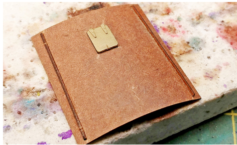
Figure 216: Here is the roof assembly. The hatch (Precision Scale Company #HO-3234) was glued in place using CA glue from the underside of the roof. The ridges were also glued into their etched locations using the same adhesive.
