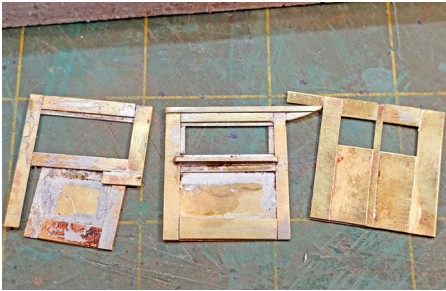
Figure 199: The window mullion, being butt soldered, didn't survive its placement in the two examples on the left. The cab side on the right had a more secure mullion, but precluded making a wooden cab side.
