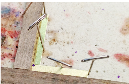
Figure 203: Shown are the two cab sides, cut from 0.024" thick cherry. The scribing for the inset wooden panel is a 3 scale inches apart and was only done on the portion that will show when placed behind the brass outer layer of the finished assemblies.
