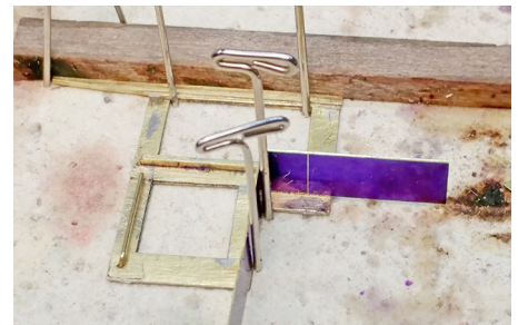
Figure 212: A simple and temporary jig was used to hold the shroud and cab side for soldering. This was before flipping the cab side over and using four pushpins to guide the shroud. I applied light pressure with the point of a needle awl to hold it in place for soldering.
